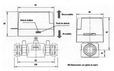
Valve position - In the event that mains power is disconnected the valve automatically spring-returns to the closed position (Port A).
