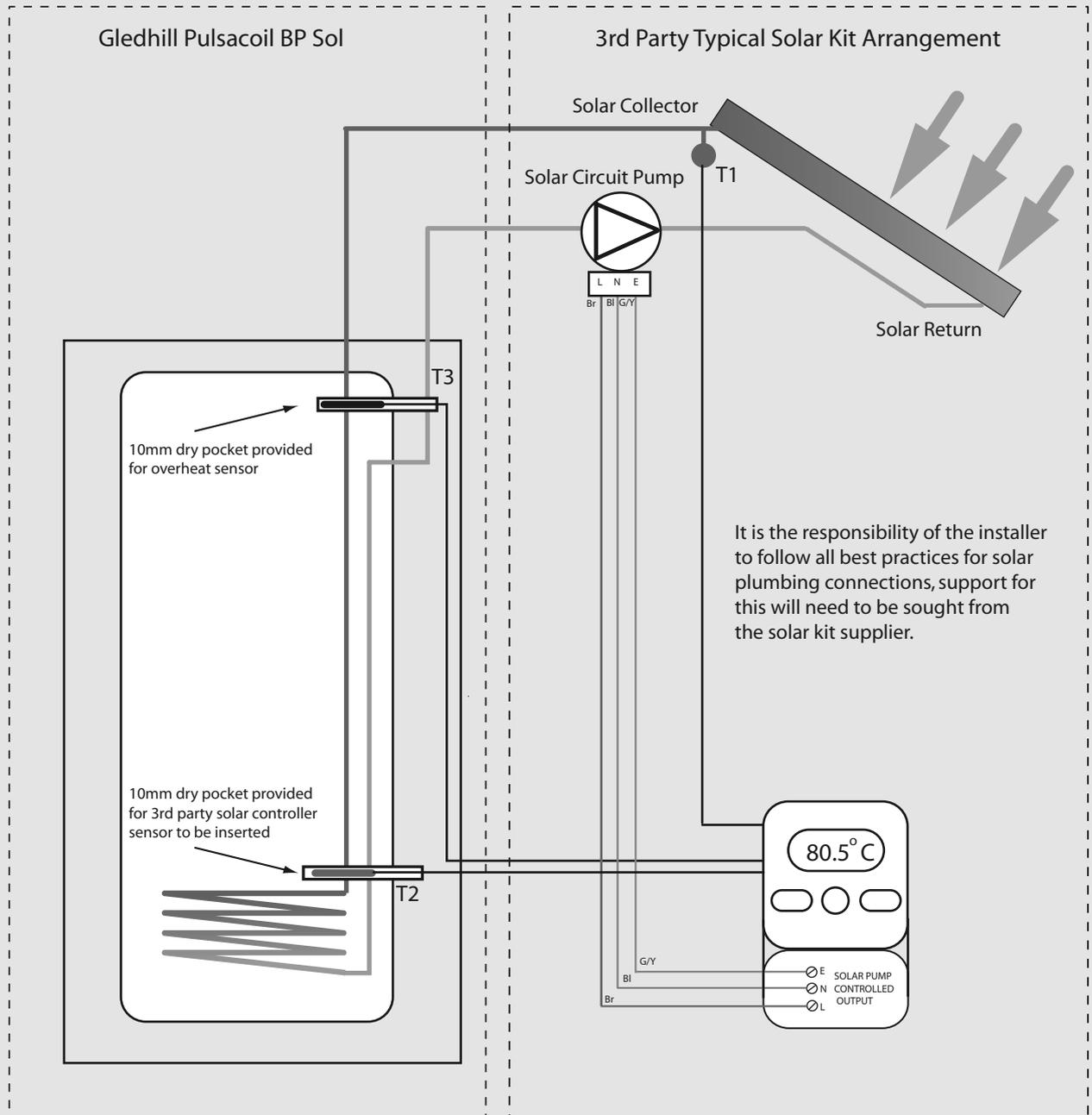
This diagram must be used in conjunction with the full Pulsacoil BP wiring diagram in the Design, Installation and Servicing Instruction Manual.
